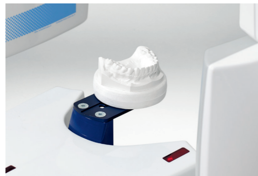
Scanning a plaster cast to a digital model
